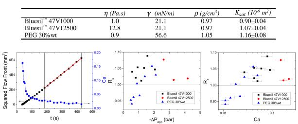
**Figure 1:** (a) Squared flow front and capillary number against time for the experiment with Bluesil<sup>TM</sup> 47V1000 at 0.46 bar. (b) Ratio  $R_s$  for all the experiments as a function of the applied pressure difference. (c) Ratio  $R_s$  as a function of the average capillary number for all the experiments.
